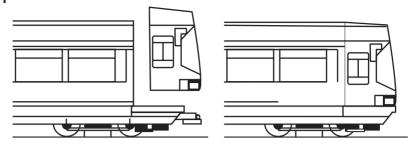
Fig. 10.30 Bonding of a front cabin to a train.
