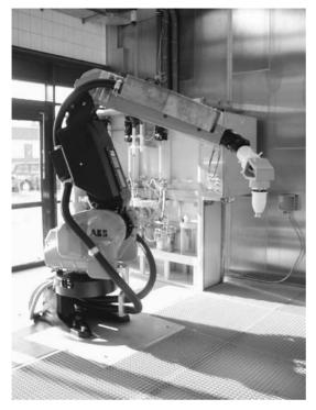
Fig. 1.5 Paint robot with electrostatic bell (source: BASF Coatings).
