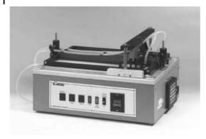
Fig. 12.81 Abrasion scrub tester (source: Byk-Gardner).
