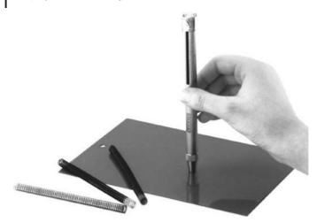
Fig. 12.63 Hardness meter (DUR-O-Test) (source: Erichsen).
