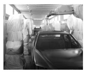
Fig. 8.36 Second application step of metallic base coats with high-speed-rotating atomizer and electrostatic paint charging.
