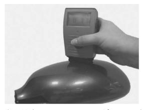
Fig. 12.16 The instrument 'microwave-scan' for orange peel and DOI measurement of small and curved parts (source: Byk–Gardner).
