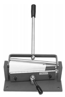
Fig. 12.71 Conical mandrel (source: Erichsen).
