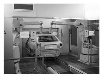
Fig. 8.30 Robot-guided contactless online measurement of film thickness.
