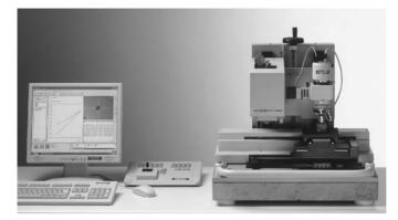
Fig. 12.62 Total hardness measurement system (source: Helmut Fischer GmbH & Co. KG).
