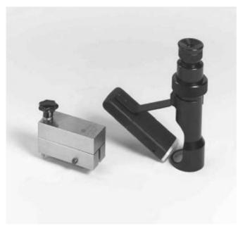
Fig. 12.60 Buchholz test equipment (source: Byk-Gardner).
