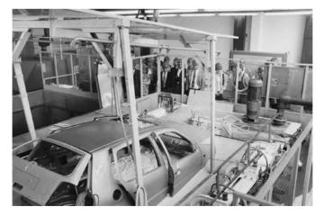
Fig. 12.54 Pilot electrocoat tank (source: BASF).
