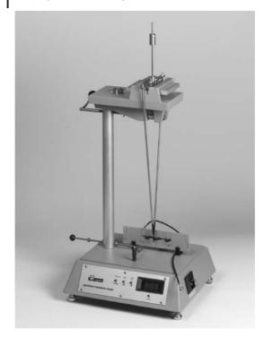
Fig. 12.59 König Pendulum damping device (source: Byk-Gardner).
