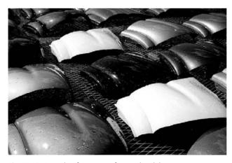
Fig. 12.39 Example of specimen for weatherability tests.
