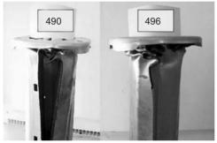
Thickness of metal sheets is about 1mm
