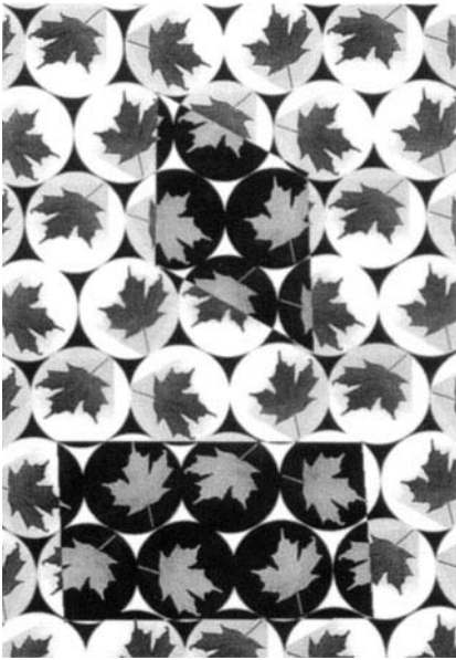
Fig. 1b. A parallelogram unit cell and a centered double unit cell for the pattern
