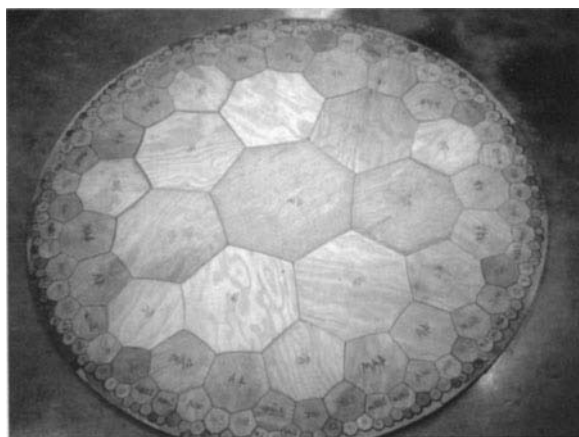
Fig. 5. To debug the water-jet program, a full set of wooden blocks was cut and then assembled
