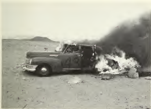
Figure 7.27. Thermal radiation from a nuclear explosion ignited the upholstery and caused fire to spread in an automobile, Nevada Test Site.
