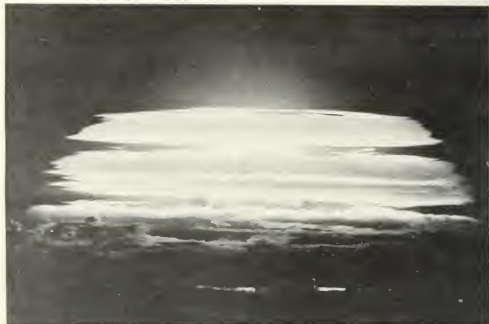
Figure 2.04. Fireball from an air burst in the megaton energy range, photographed from an altitude of 12,000 feet at a distance of about 50 miles. The fireball is partially surrounded by the condensation cloud (see § 2.48).
