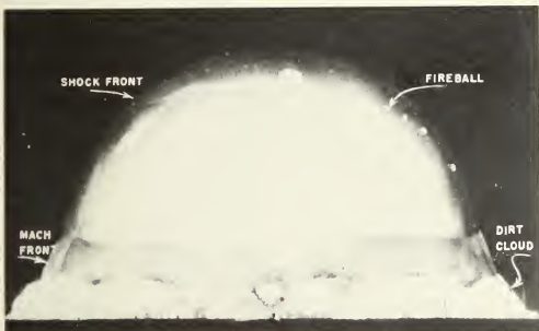
Figure 2.32. The faintly luminous shock front seen just ahead of the fireball soon after breakaway (see § 2.120).
