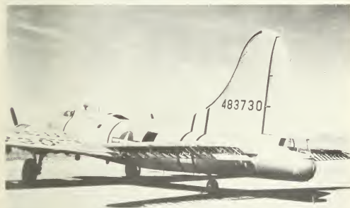
Figure 5.95b. Aircraft after tail exposed to a nuclear explosion (2.4 psi peak overpressure).
