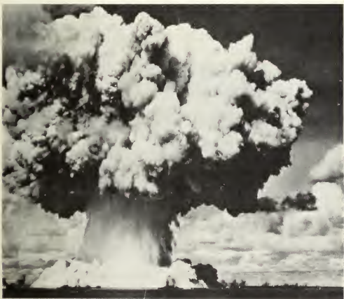
Figure 2.68. The radioactive cloud and first stages of the base surge following a shallow underwater burst. Water is beginning to fall back from the column into the lagoon.
