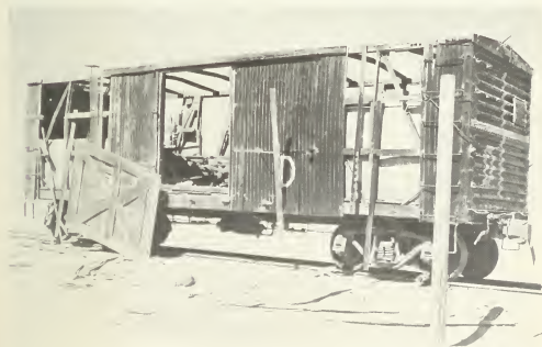
Figure 5.92b. Loaded wooden boxcar after a nuclear explosion (6 psi peak overpressure).
