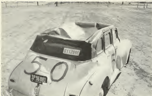
Figure 5.87a. Damage to automobile originally located behind wood-frame house (5 psi peak overpressure); the front of this car can be seen in Figure 5.57. Although badly damaged, the car could still be driven after the explosion.
