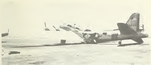
Figure 5.95a. Aircraft after side exposed to a nuclear explosion (3.6 psi peak overpressure).
