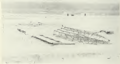
Figure 5.51b. Structure similar to Figure 5.48b after exposure to 5 psi peak overpressure and 0.5 psi dynamic pressure; positive phase duration several seconds.
