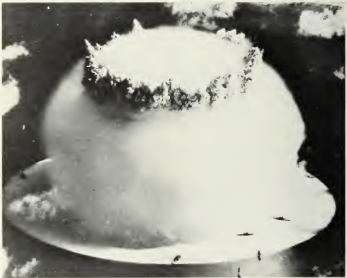
Figure 2.67a. The condensation cloud formed after a shallow underwater explosion. (The "crack" due to the shock wave can be seen on the water surface.)
