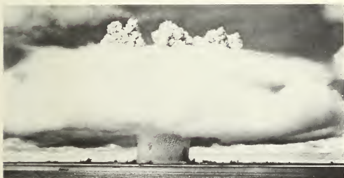
Figure 2.67b. Formation of the hollow column in a shallow underwater explosion; the top is surrounded by a late stage of the condensation cloud.
