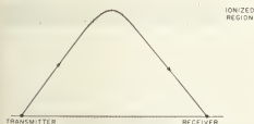
Figure 10.08. Reflection of a radio (or radar) wave by successive refractions in an ionized region of the atmosphere.
