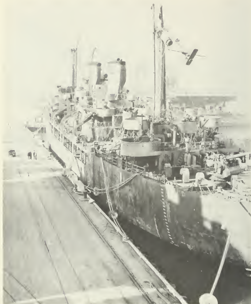
Figure 5.96. The U.S.S. Crittenden after ABLE test; damage resulting was generally serious (0.47 mile from surface zero).
