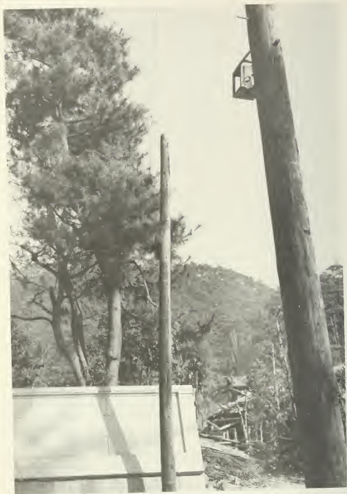
Figure 7.63. The top of a wood pole was reported as being ignited by the thermal radiation (1.25 miles from ground zero at Hiroshima, 5 to 6 cal/cm 2 ). Note the unburned surroundings; the nearest burned building was 360 feet away.
