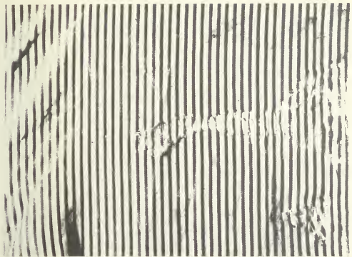
Figure 7.48. The light-colored portions of the material are intact, but some of the dark-colored stripes have been destroyed by the heat from the thermal radiation.
