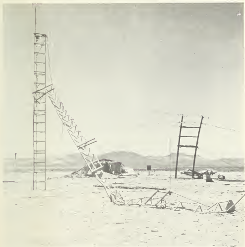
Figure 5.124. Unguyed lightweight 120-foot antenna tower (5 psi peak overpressure, 0.6 psi dynamic pressure from 30-kiloton explosion), Nevada Test Site.
