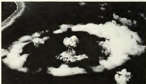
Figure 2.50. Late stage of the condensation cloud in an air burst over water.
